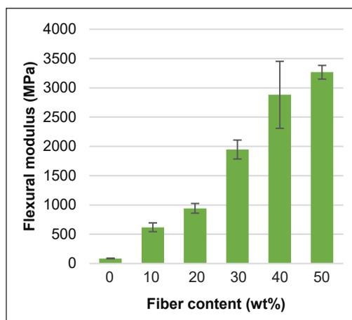
Figure 8. Flexural modulus of TPS/Beeswax + coconut fiber
