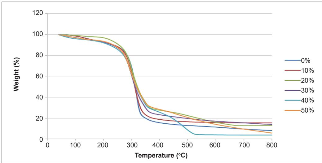
Figure 3. TGA curve of TPS/Beeswax + coconut fiber composite
