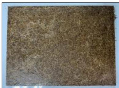
Figure 2. TPS/beeswax reinforced with coconut fiber
