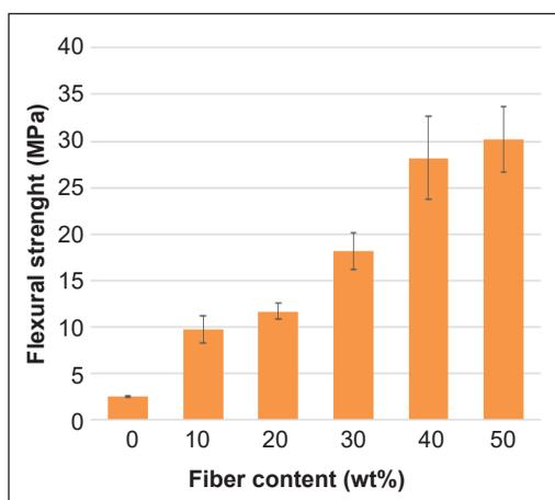
Figure 7. Flexural strength of TPS/Beeswax + coconut fiber
