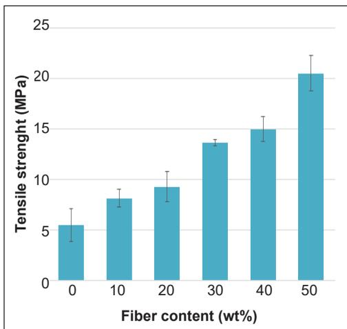
Figure 5. Tensile strength of TPS/Beeswax + coconut fiber
