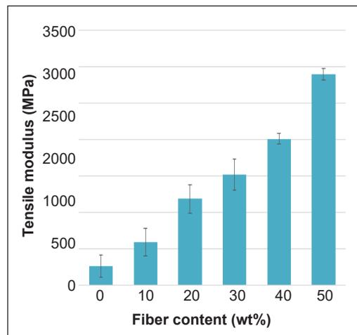
Figure 6. Tensile modulus of TPS/Beeswax + coconut fiber
