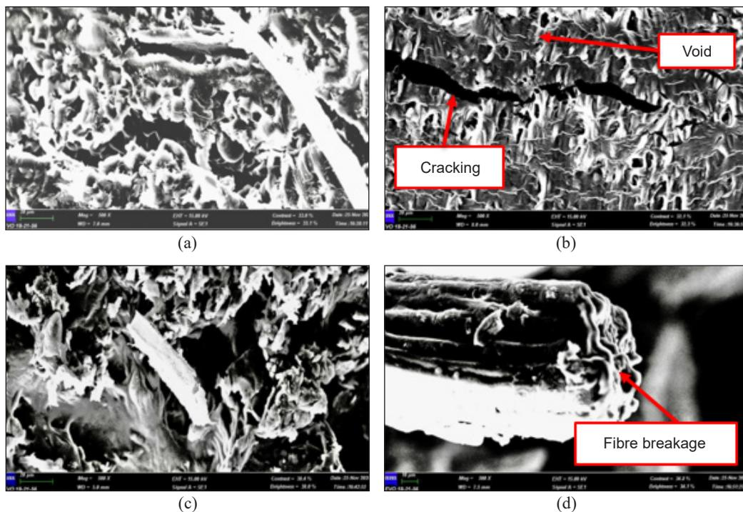
Figure 10. SEM micrograph of a fracture surface of TPCS/Beeswax + coconut fiber composites: (a) 10% fiber; (b) 20% fiber; (c) 30% fiber; and (d) 50% fiber
